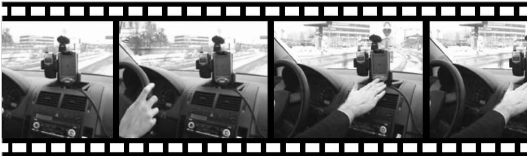
**Figure 5.** The video sequence shows the placing of a memo using a hardware button on the device. Bumps in the road cause the user to use the instrument panel as support when aiming at the button. The user lets the finger rest on the button until the right moment for pressing it occurs.
