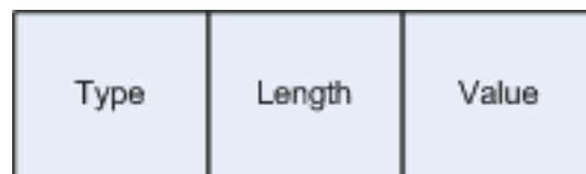
Figure 3.2: A block diagram describing the ASN.1 value encoded with BER
