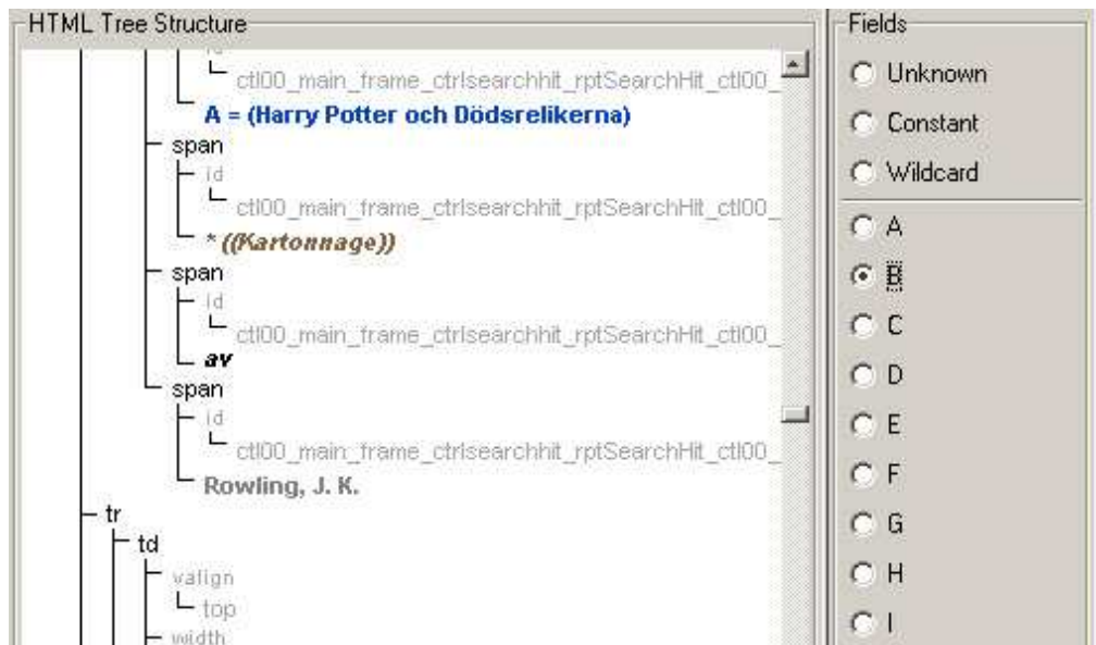
Figure 6.1: The user labeling properties of a book at www.adlibris.se . The title is labeled as variable A, the book cover is labeled as a wildcard and the word “av” (of) is labeled as a constant since it helps to identify structure in the document.
