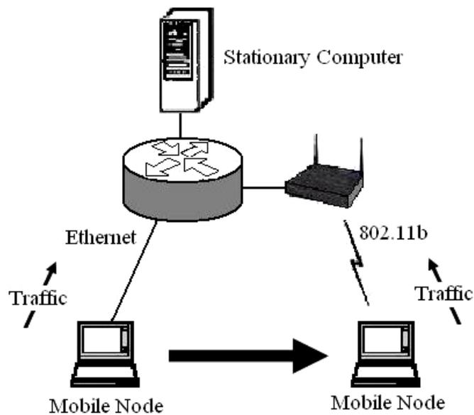
Figure 25: Testbed used in vertical handover experiments
