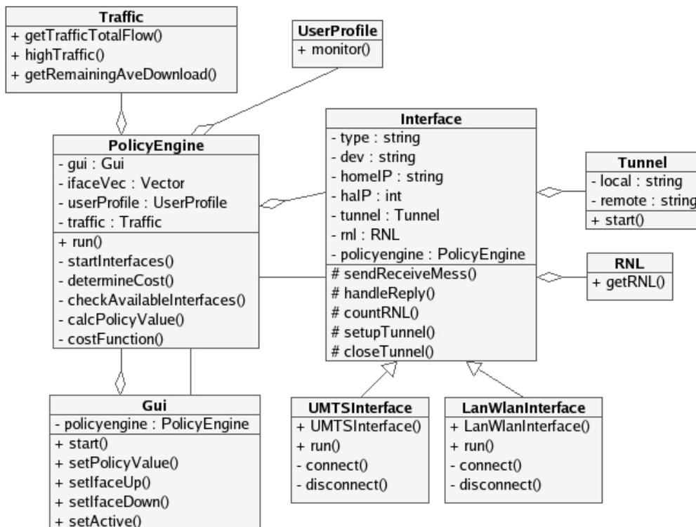
Figure 20: Class diagram for SEMO's Mobile Node application.
