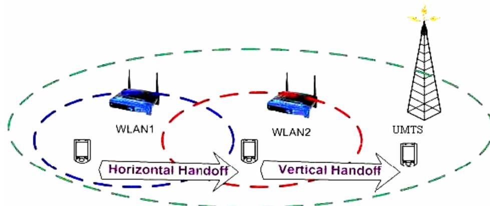
Figure 2: Horizontal and vertical handover [1]
