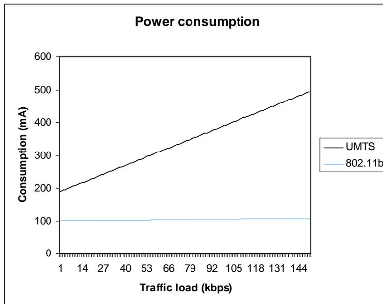
**Figure 14: Calculated traffic load and power consumption relation based on values from table 3.**
