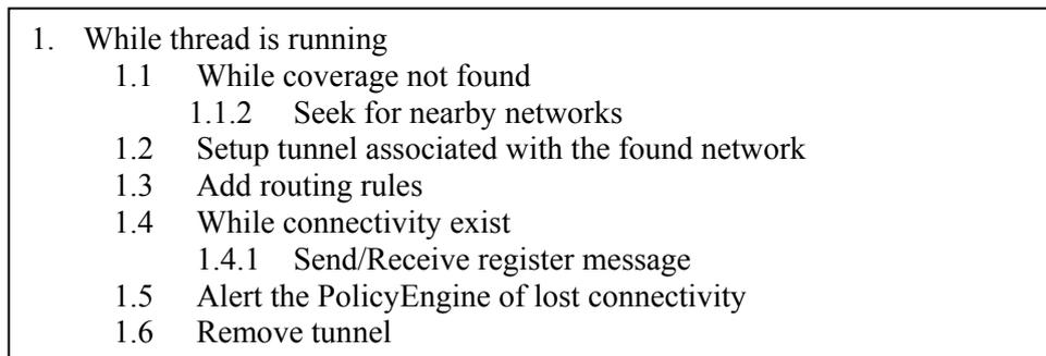
**Figure 21: Algorithm that manages connectivity aspects for an interface.**
