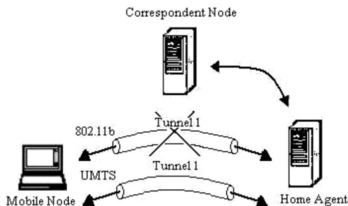
Figure 9: Hard handover from an 802.11b network to a UMTS network.
