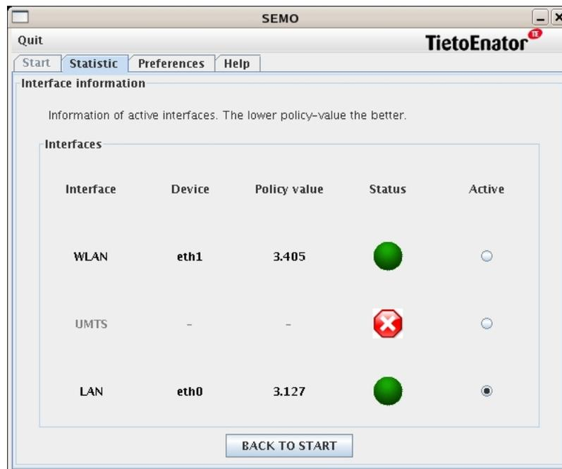
**Figure 32: Monitor network interfaces.**
