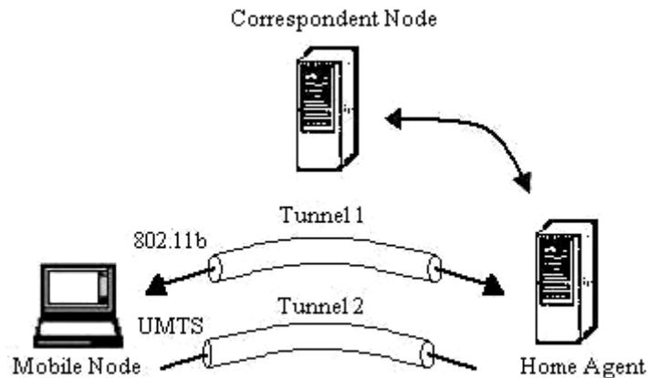
**Figure 10: One tunnel associated with each network interface.**
