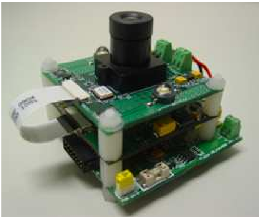
Figure 2.4: Illustration of camera stack formed from Fleck™ mainboard, DSP board and CCD camera board.
