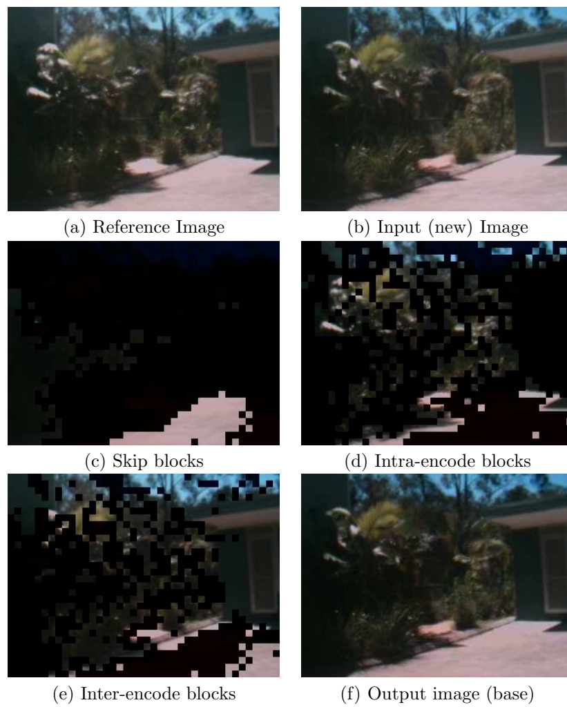
Figure 3.5: Illustration of ways in which blocks are encoded to send data.
