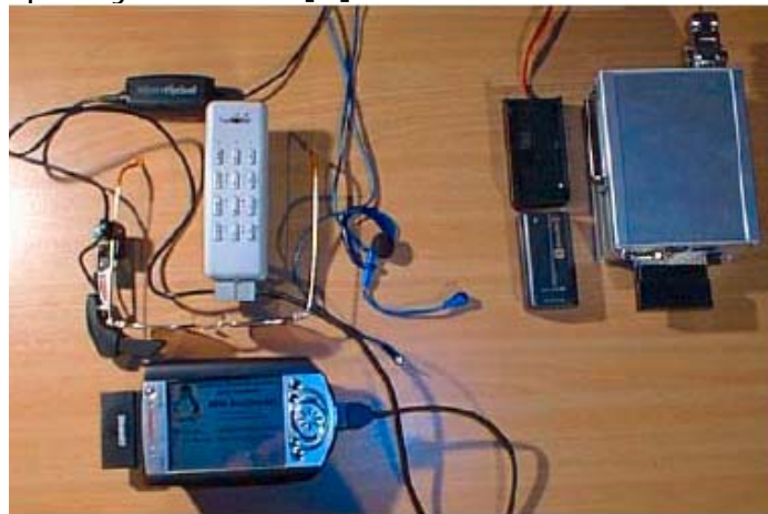
Figure 2.3: IPAQ wearable and MIP 520 wearable (right) that can work together in a WLAN-coupled body area network [6].
