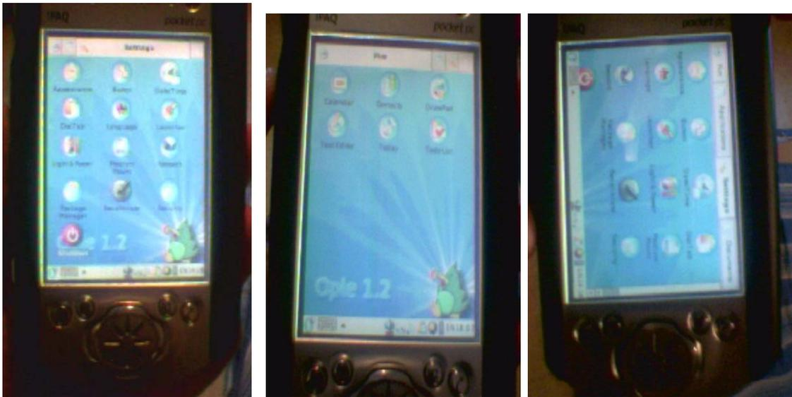
**Figure 5.4 (Linux running successfully on IPAQ 3750)**
