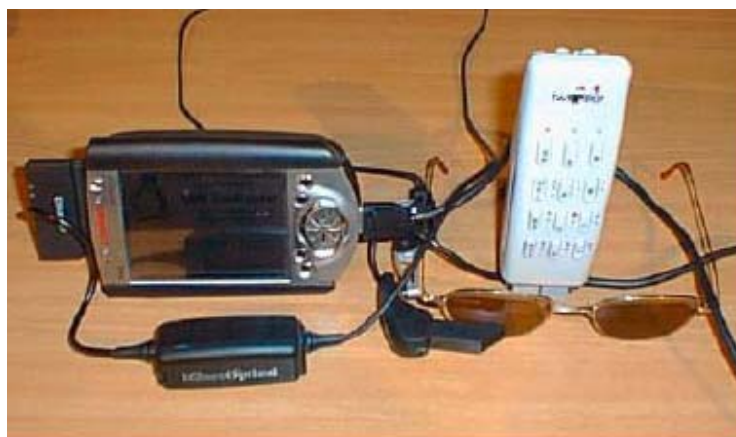
Figure 2.2: iPAQ wearable with Micro Optical head mounted display and head key twiddler chording keyboard [6].
