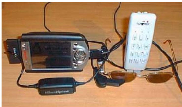
Figure 2.2: iPAQ wearable with Micro Optical head mounted display and head key twiddler chording keyboard [6].
