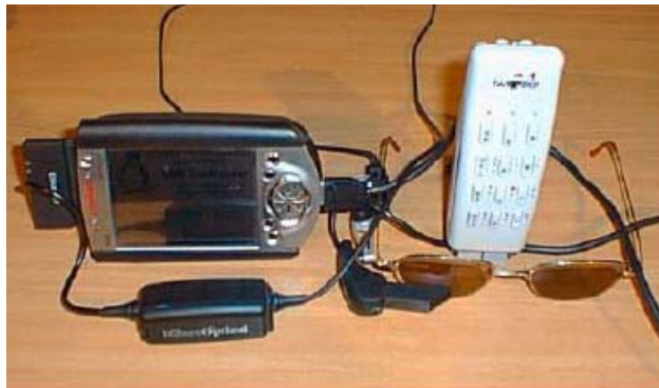
Figure 4.1: The second generation iPAQ-based wearable computer [6], with Linux in it and sensors/IO devices attached to it.
