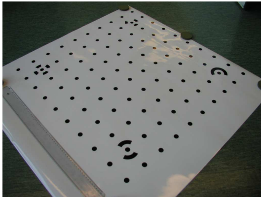
Figure 14: Example of a calibration object where four of the control points are coded.
