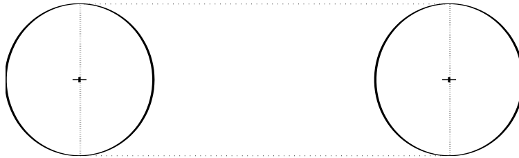
Figure 9: Common tangents to two equally sized circles
