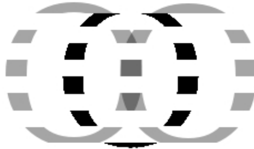
Figure 4.4: The letter 'O' is traveling from left to right. The position of the letter in three fields is shown and this is all the data used to perform the deinterlacing. In the dark gray area overlap occurs which may fool the motion detection algorithm that the pixels are stationary
