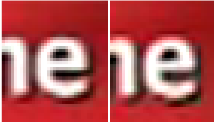
Figure 5.9: Left image is the (manually scaled) original and right is created by a previous version of the algorithm described in this Master's thesis. The right hand image has an unwanted artifact in the form of a gray shade in the bottom right corner of letter e
