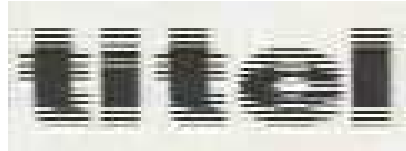
Figure 5.7: An example still frame from an interlaced clip of rolling (vertically scrolling) text
