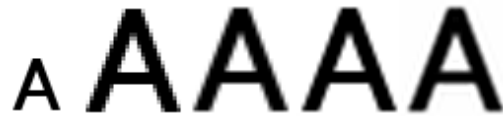
Figure 4.7: Nearest, Linear, Cubic and Lanczos scaling by a factor of 2 as implemented in GIMP
