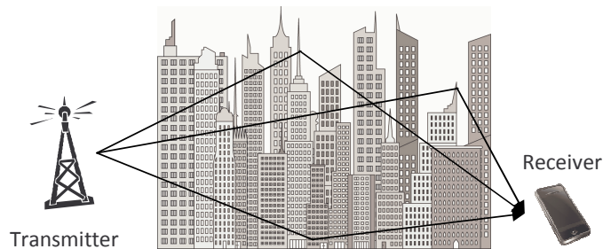
Figure 2.4: The signal sent through the wireless channel between the transmitter and receiver experience multipath fading.
