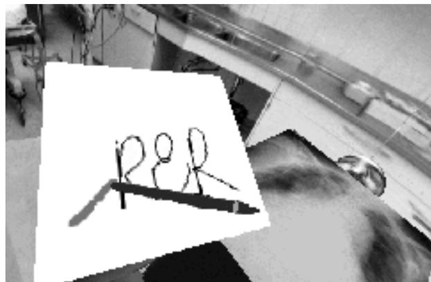
Figure 3. Pen strokes can be removed by wiping an “eraser” over them. The red line indicates the path of the eraser on the notepad.
