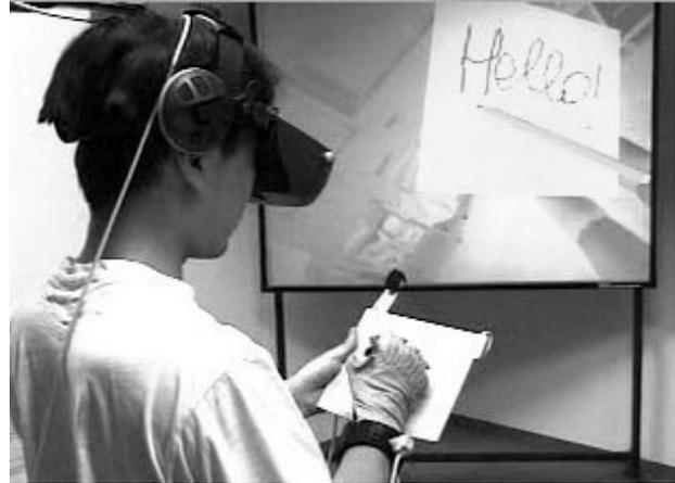
Figure 1. The physical setup of Virtual Notepad. The user is provided with a spatially-tracked tablet and pen for taking notes in the VRER.
